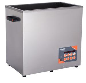
\* Special stainless steel tank made in AISI 316Ti thickness 20/10 with round tank corners for a better removing of dirt residuals after cleaning process. The tank is welded with TIG process
