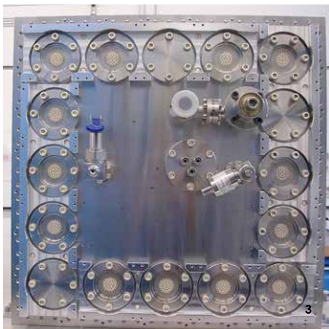
Figura 3 - MWPC Detector: back flange (Steel)
