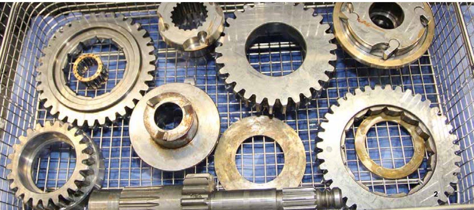
Figure 2 - Winch parts before ultrasonic treatment
