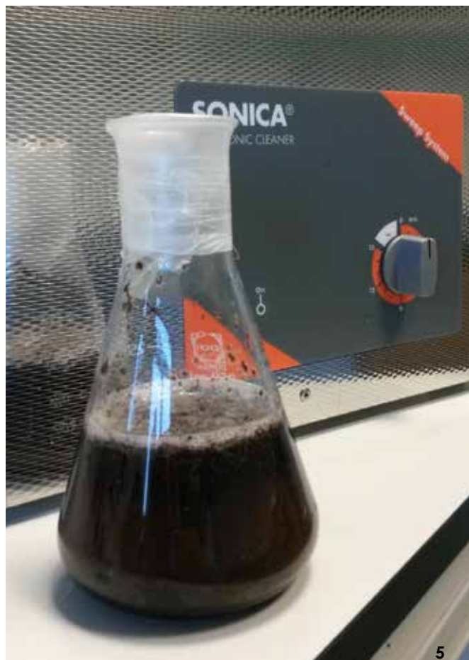
Figure 5 - Glass flask after ultrasonic extraction with Sonic a Bath
