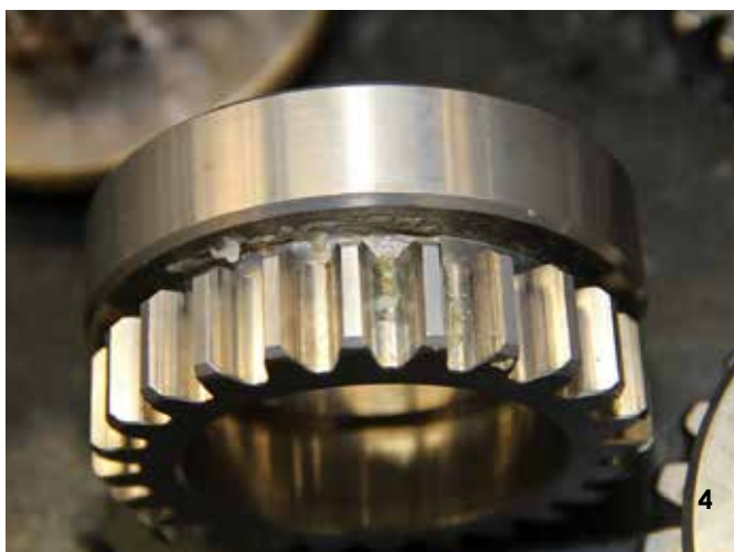
Figure 1/3/4 - Details with obvious signs of dirt and oxidation before ultrasonic treatment
