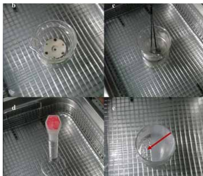
Figure 3 - Cleaning in Ultrasonic Bath SONICA 3200 EP: a) Ultrasonic Bath SONICA 3200 EP, b) STM electrochemical cell, c) tweezers, d) glassware, e) glue used for coating of the tips.
