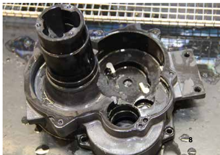
Figures 7/8 - Detail before and after ultrasonic treatment
