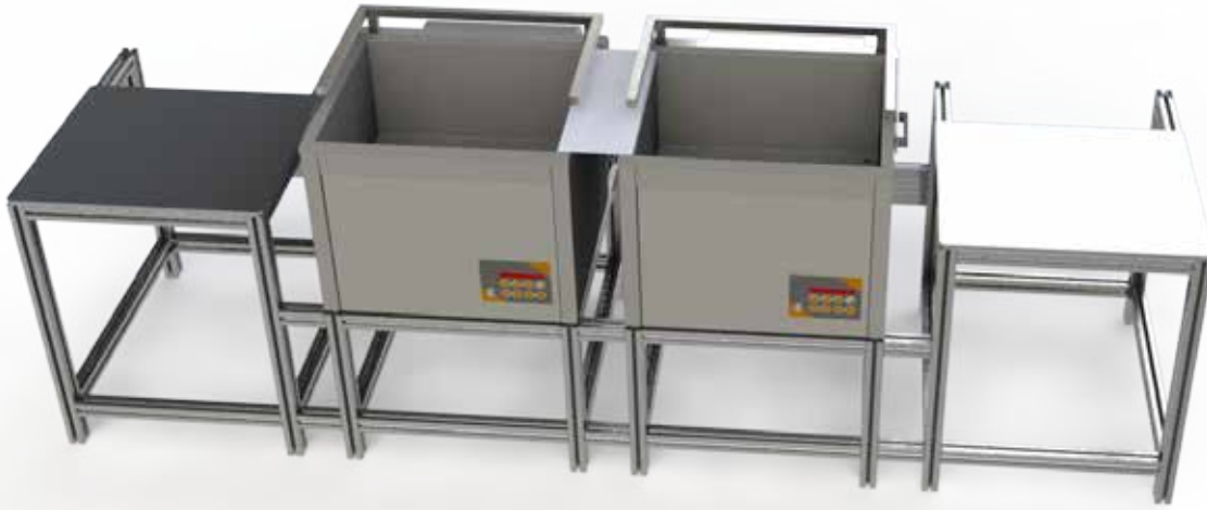
Figure 3 - New modular system with automatic oscillating movement of the basket
