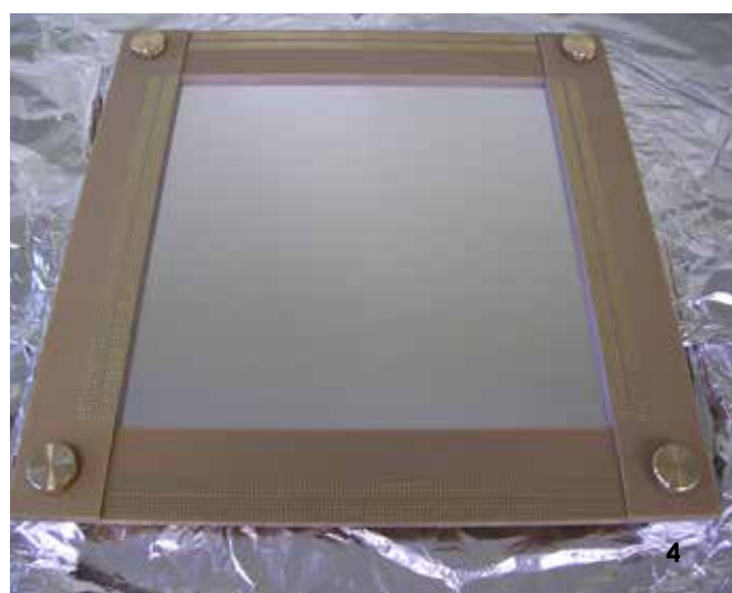
Figure 4 - MWPC Detector: PCB
